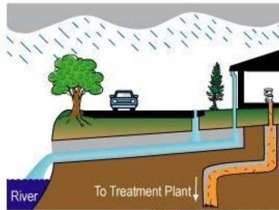
Figure 4-4: Separated wastewater system
