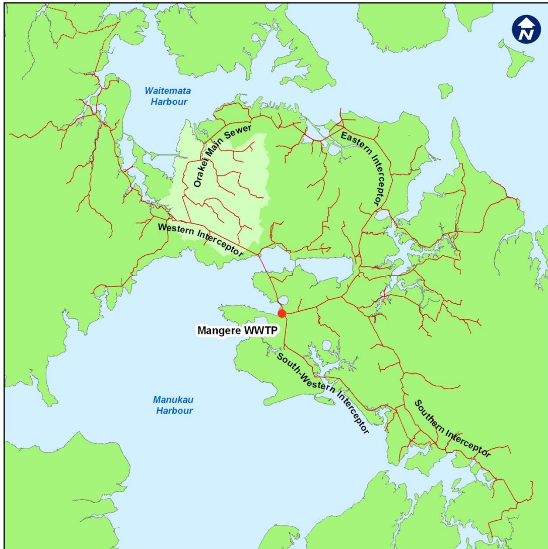
Figure 3-2: Wastewater network delivering flow to Mangere WWTP (Central Interceptor catchment area shaded)
